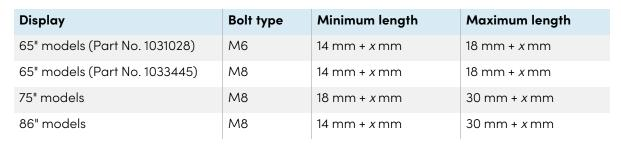
where x is the combined thickness of the wall mount and washer
